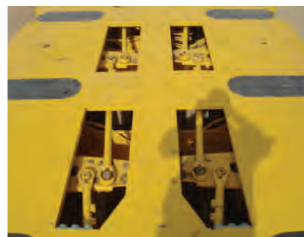
The connecting rods of a mechanical steering system seen through the openings in the deck
