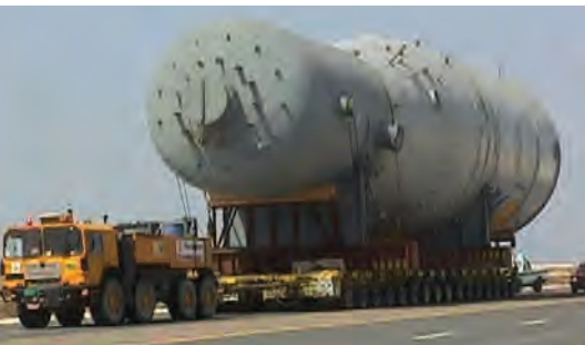
A pull type transport with prime mover and drawbar
