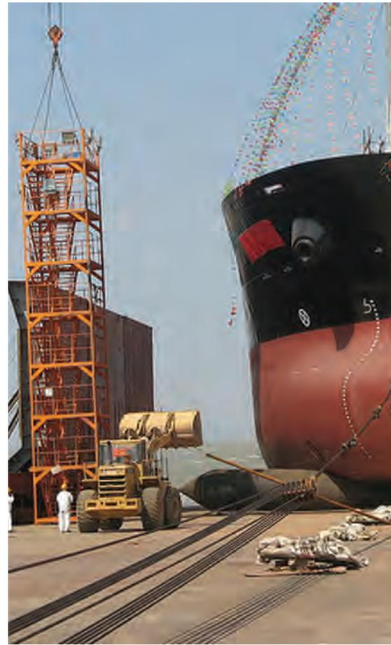
Disadvantages are the inability to make corrections during the launch and the necessity of building the vessel in front of or on a launch ramp. If the ship building company is building multiple vessels at the same time, they will need multiple launch ramps. The picture above shows an airbag launch where the airbags can still be seen on the bow of the vessel. The tie back arrangement can also be seen.
