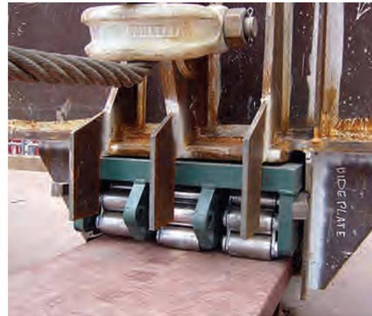
A group of tank rollers on a steel guide track
