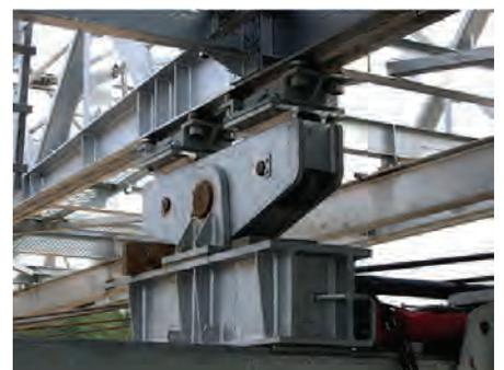
Tank rollers to reduce friction in heavy shift applications
