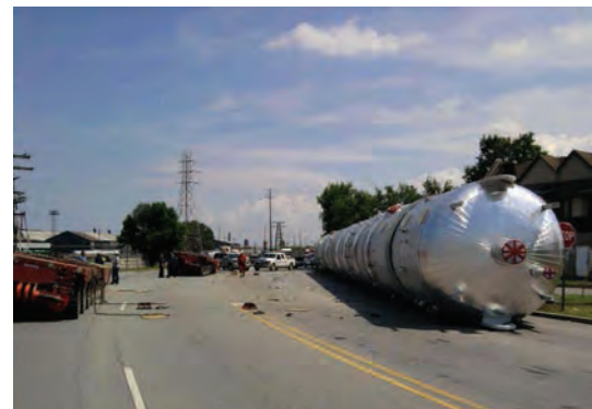
Avoiding an accident with a dolly load requires attention to be paid to maintaining equal velocity of the dollies
