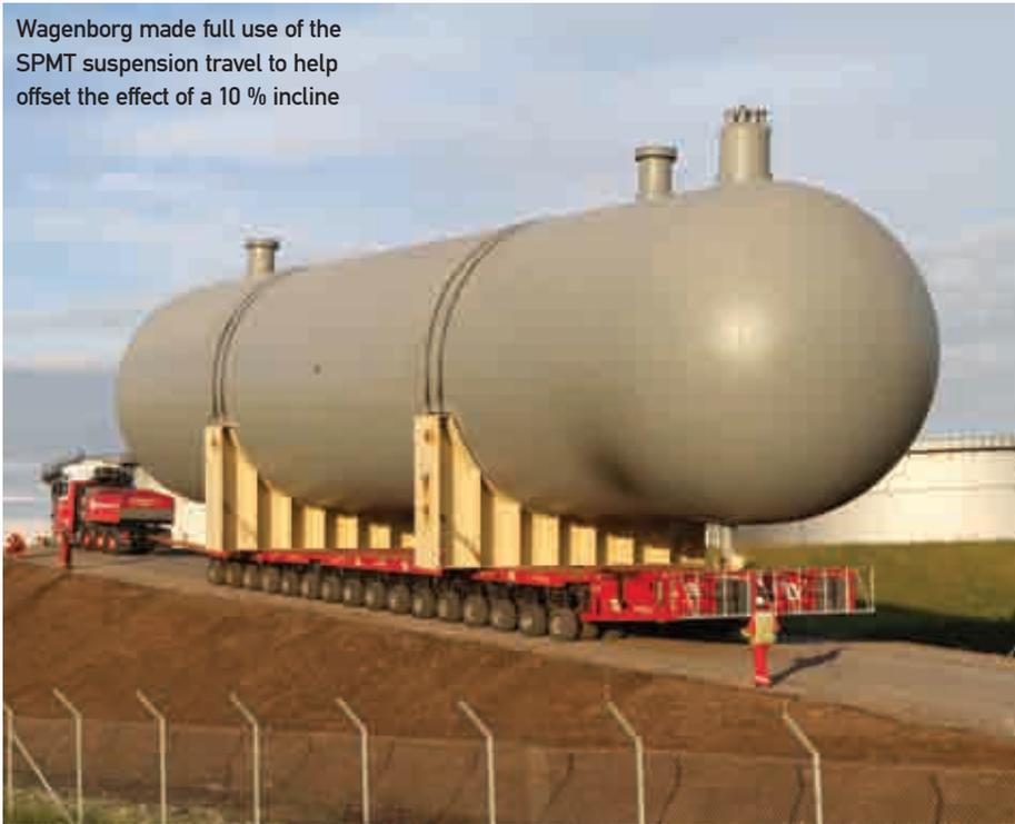
12.2 degrees, sufficient to carry out the transport in a safe manner.
