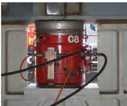
FIGURE 4 Load cell in application with Mammoet on a hydraulic jack
